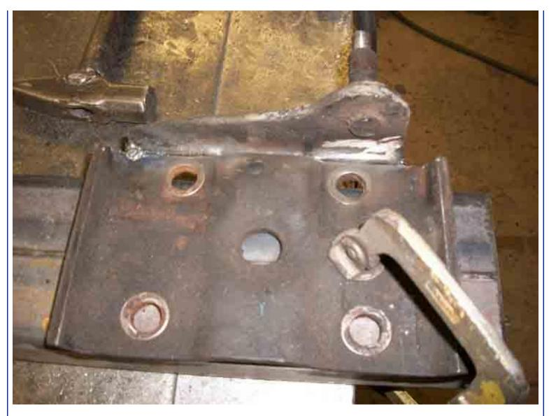
Weld it up on both sides (make sure that the area where the hardened washer sits is flat, grind if needed).
